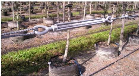
Turnbuckles are inexpensive, but essential for tightening the system and occasionally adjusting tension.
